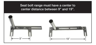
No matter what orientation you choose, the lower pole must be positioned closest to the front inner corner of the passenger seat against the console/transmission hump.
