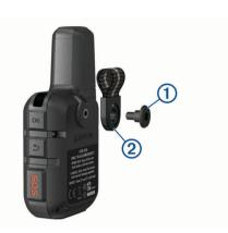
2 Secure the spine mount adapter ① over the back of the device using the long screw ② included with the device.
