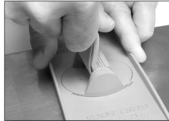
After the strap has been tightened, lift it up and hold **together** with the tab.
