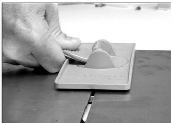
Firmly holding the strap and the tab, lower them in the direction of the strap to lock the Gust Lock.
