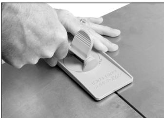
Holding Gust Lock firmly in place, tighten the strap.
