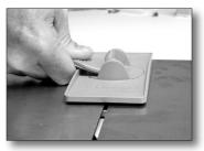
Firmly holding the strap and the tab, lower them in the direction of the strap to lock the Gust Lock.
