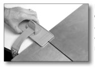
Make sure that both parts of the wing are aligned flat and slide on the Gust Lock to cover the split between two surfaces.
