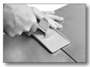
Holding Gust Lock firmly in place, tighten the strap.
