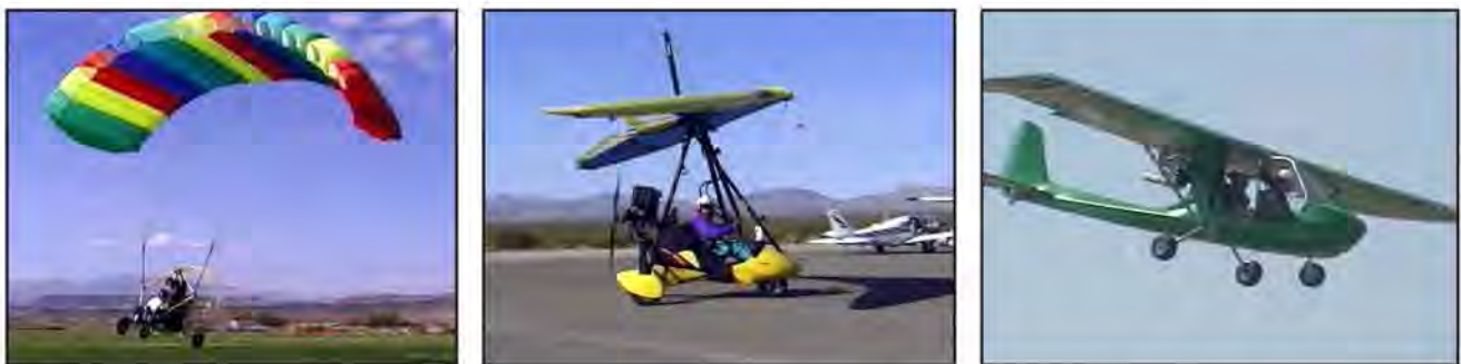
Figure 1-3. The powered parachute has some unique operating characteristics as compared to other light-sport aircraft. Left, PPC with inflated wing; middle, weight-shift control aircraft; right, fixed-wing LSA.
