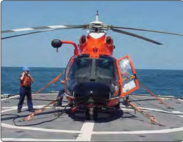
Figure 1-13. Example of mooring of a helicopter.
