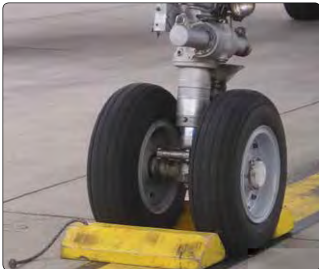
Figure 1-12. Wheels chocked fore and aft.
