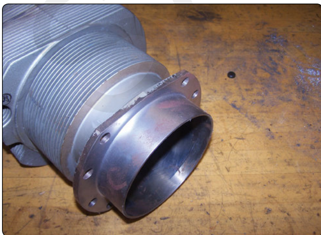
Figure 1-18. The aluminum head and steel barrel of a cylinder.
