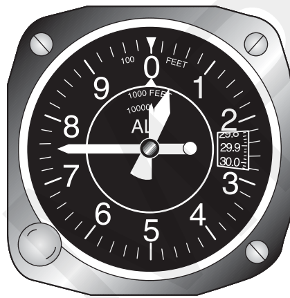
Figure 4-4. An altimeter measures absolute pressure and displays it as feet of altitude above the pressure reference level that has been set into the barometric window.
