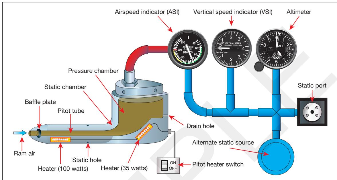
**Figure 5-3.** Pitot-static system and instruments. (FAA Pilot's Handbook of Aeronautical Knowledge)
