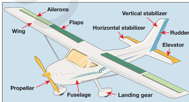
Figure 4-7. Parts of a small aircraft.
