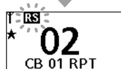
When no reply signal is received, automatically accesses the next repeater.
