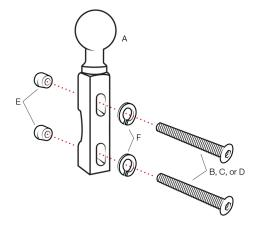
While holding factory clamp assembly in place, remove second factory bolt and replace with RAM® Base with hardware from Step 1. Store any unused components or hardware for possible future use.
