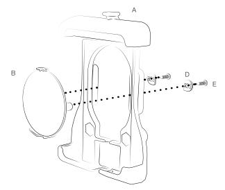
Shift Apple MagSafe cable up and down until magnets are properly aligned with phone. Once aligned, fully tighten (E) Screws on the back. Hand-tighten only, do not over-tighten.
