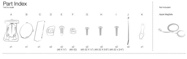
Connect (B) Puck Slide to (A) RAM<sup>®</sup> Quick-Grip<sup>™</sup> Holder, using (E) Screws and (D) Ratchet Washers. Do not fully tighten yet.
