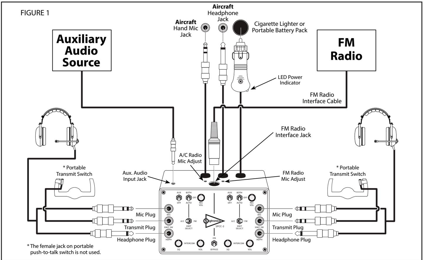
aircraft does not have either one of these jacks, they can be installed by any qualified avionics technician. If you plan to use the SPCC in a helicopter, please contact Sigtronics for advise on adapting the general aviation plugs to the helicopter jacks.
