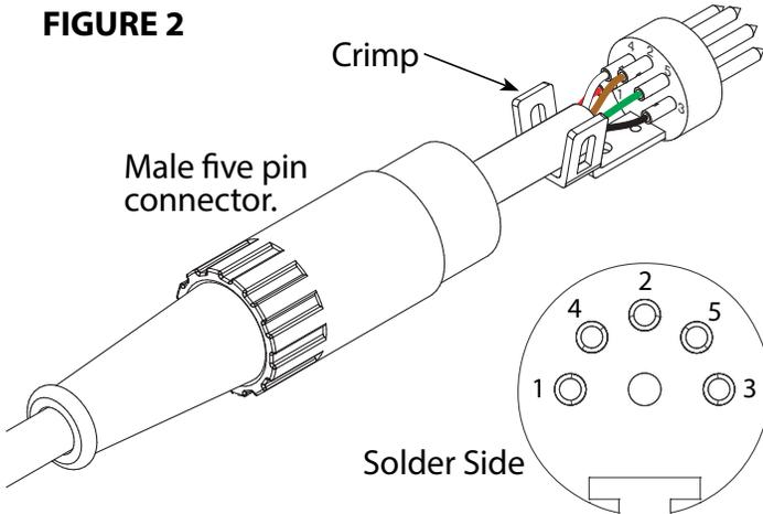
**FM RADIO INTERFACE CABLE WIRING**
