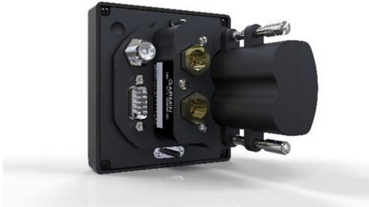
Figure 1-2 G5 Standby Battery
