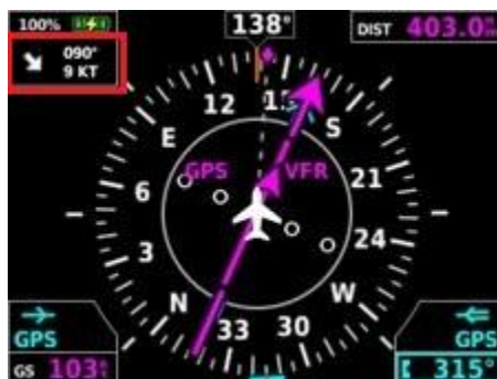
Figure 6-5 HSI Display of Crosswind (Typical Values Shown)
