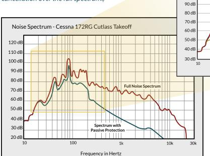
In this close-up of only low frequency noise, the red line shows a noticable reduction in the additional attenuation provided with active cancellation over a typical passive headset. Understand that there will be a slight reduction in higher
