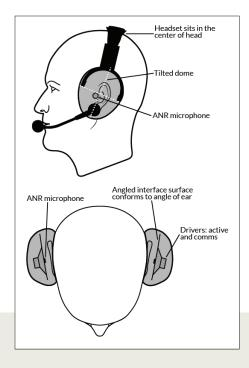
Domes are tilted and shaped for a better fit, and the mounting plates for the mic and speaker are angled to follow the ear's profile. These ergonomic and acoustic details significantly improve both comfort and performance.
