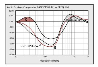
All of the tested headsets show declining cancellation at frequencies above 300 Hz. The deeper the 100 Hz cancellation, typically the steeper the profile drops off between 300 and 600 Hz. The steeper the drop-off, the harder it is to avoid some "overshoot" of uncancelled noise.
