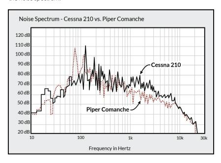
Actual noise data measured during flight in two different single-engine airplanes: a Cessna 210 and a Piper Comanche.
